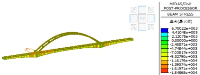
Fig.6 Stress Diagram of Main Beam and Arch Rib.
